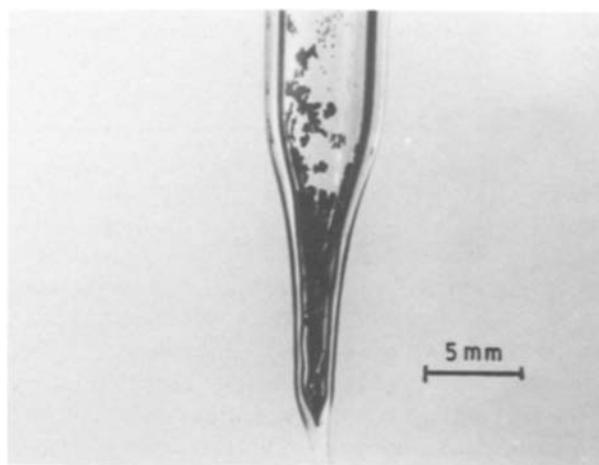
Figure 3 Needles emerging from the tip of the pointed end of the ampoule (temperature difference  $50^{\circ}\text{C}$ ).
