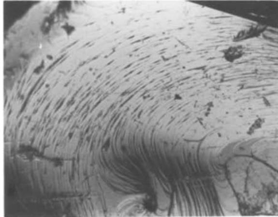
Figure 5 Step-like layers,  $\times 800$ .
