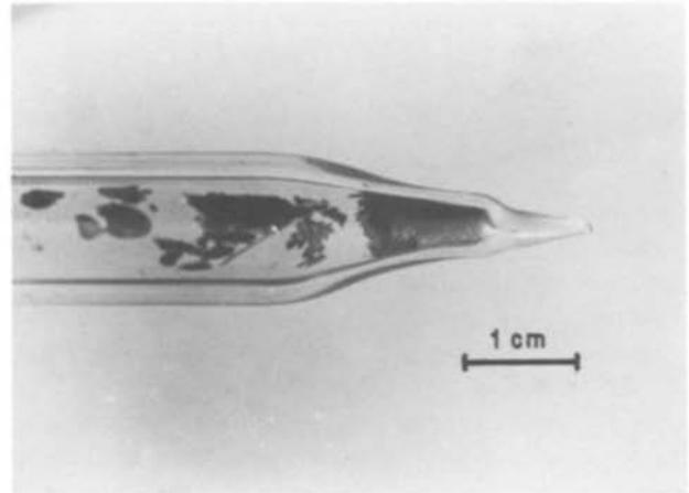
Figure 8 BiSeI boule (growth temperature  $510^{\circ}\text{C}$ ).
