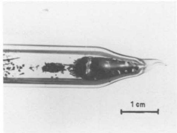
Figure 7 Platelets of BiSeI (growth zone temperature  $520^{\circ}\text{C}$ ).
