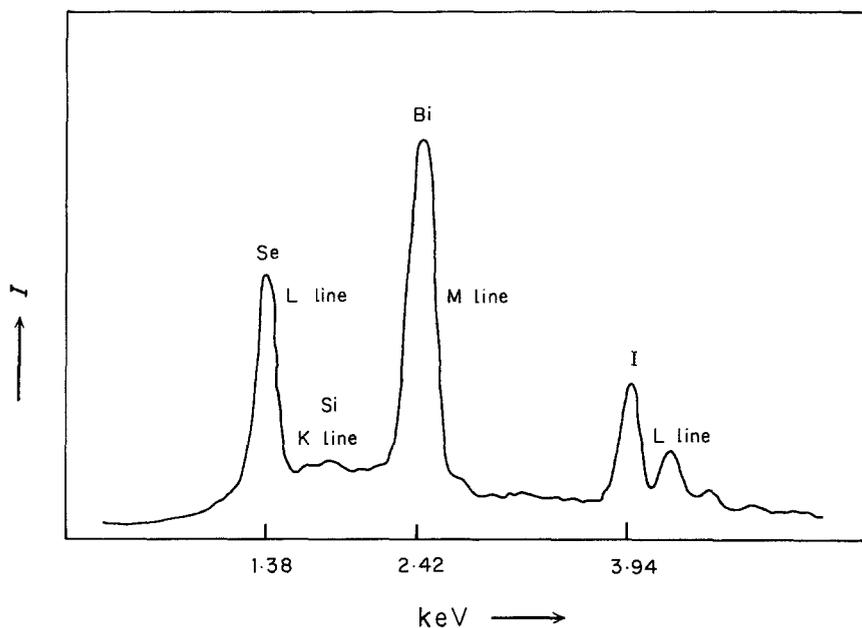
Figure 10 Spectral analysis of BiSeI crystals.
