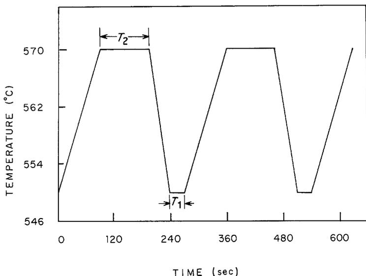
Figure 1 Time-temperature plot for the oscillation method.
